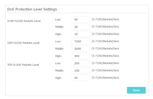
**3.** Configure ICMP-FLOOD Attack Filtering, UDP-FlOOD Attack Filtering and TCP-SYN-FLOOD Attack Filtering.
