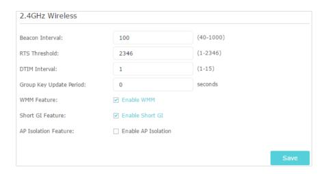
Beacon Interval - Enter a value between 40-1000 milliseconds for Beacon Interval here. Beacon Interval value determines the time interval of the beacons. The beacons are the packets sent by the router to synchronize a wireless network. The default value is 100.
