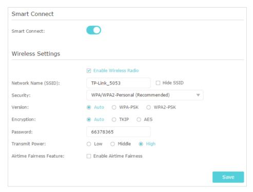
3. Keep the default or set a new SSID and password, and click Save. This SSID and password will be applied both for 2.4GHz and 5GHz wireless networks.
