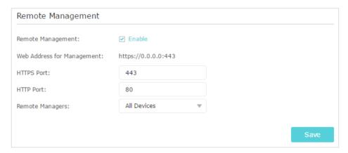
Devices on the internet can access manage the router via the Web Address for Management, such as https://0.0.0.0:43 shown.
