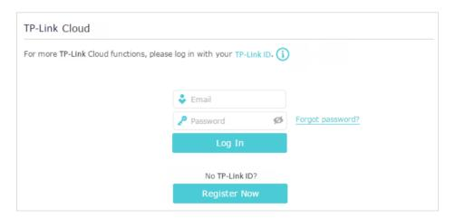
4. After activating your TP-Link ID, come back to the TP-Link Cloud page to log in. The TP-Link ID used to log in to the router for the first time will be automatically bound as an Admin.
